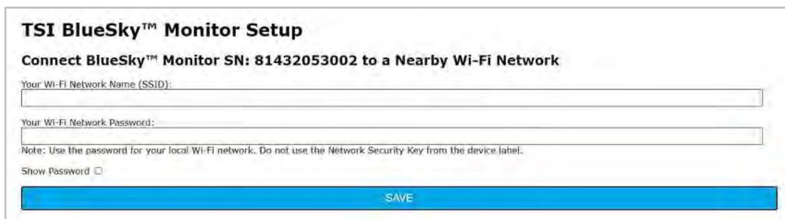
**Figure 10:** Entering Wi-Fi network SSID and password
