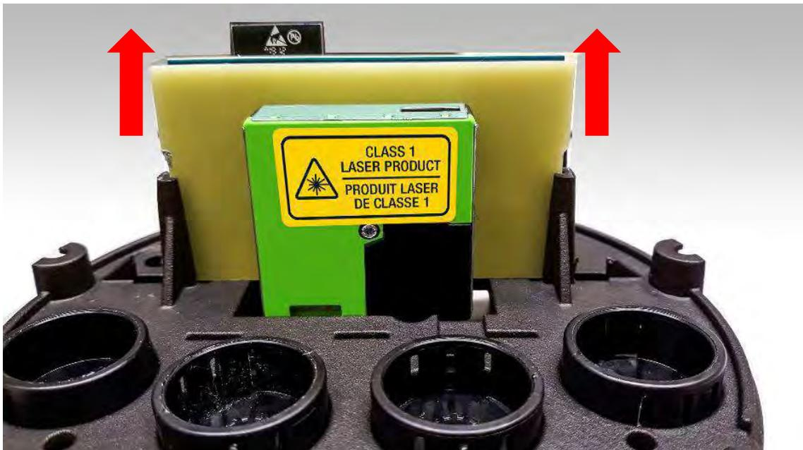
**Figure 27:** Replacing PM sensor
